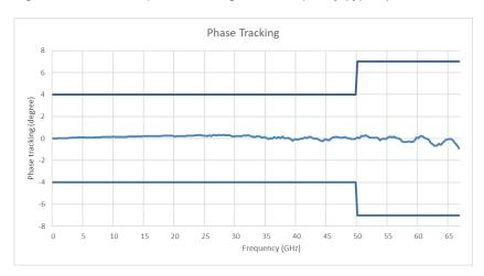
Figure 18. 11667D phase tracking versus frequency (typical)
