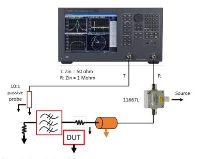
Figure 3. Non- 50-ohm LF filter measurement
