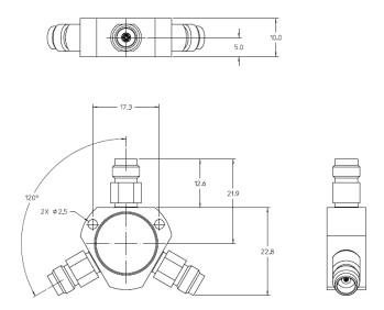
Figure 22. 11667C/D mechanical dimension
