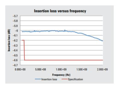
Figure 8. 11667L insertion loss versus frequency (typical)
