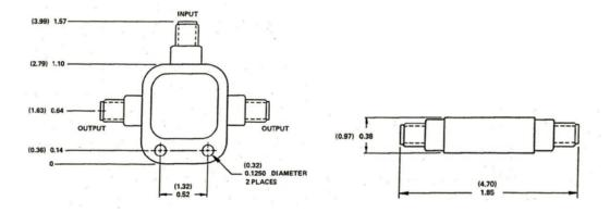
Figure 21. 11667B mechanical dimension
