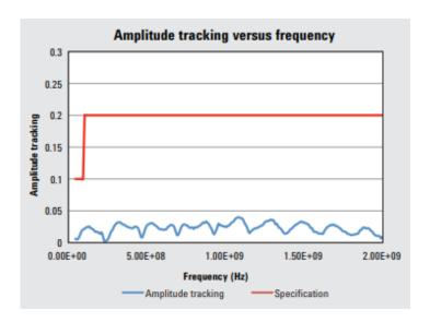
Figure 10. 11667L amplitude tracking (dB) versus frequency (typical)
