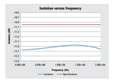
Figure 9. 11667L isolation versus frequency (typical)
