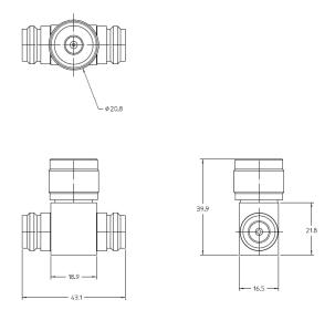
Figure 20. 11667A mechanical dimension
