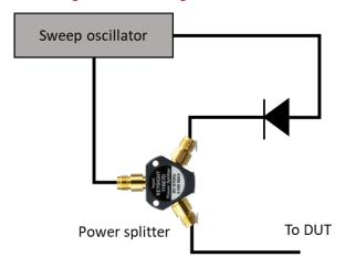
Figure 4. Power splitter test setup for leveling with a crystal detector
