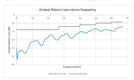
Figure 15. 11667D Output equivalent return loss versus frequency (typical)
