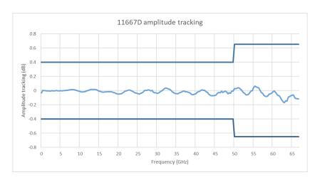
Figure 17. 11667D Amplitude tracking versus frequency (typical)
