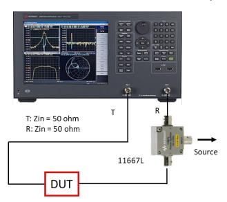
Figure 2. 50-ohm device measurement
