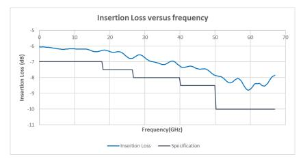
Figure 16. 11667D Insertion loss versus frequency (typical)
