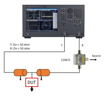
Figure 1. Shunt-thru impedance measurement
