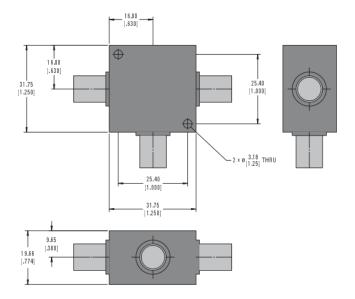
Figure 19. 11667L mechanical dimension
