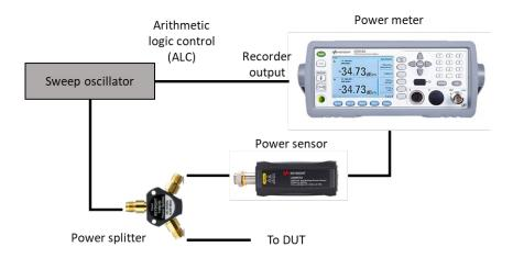
Figure 5. Power splitter test setup for leveling with a power meter
